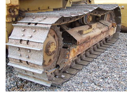
Figure 6: The moving caterpillar track on a bulldozer.
